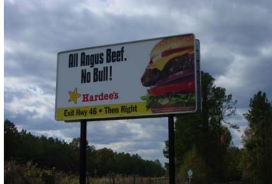
For this reason, the overall size of the finished vinyl is extremely important. The overall finished size should be 10’-7” x 22’-10” including the pockets. If this size is exceeded, the vinyl will be too large for the panel and cannot be fully tightened.
